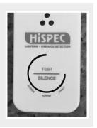
While the red I FD is lit on the first alarm, to add other CO alarms to the Home Group, take one from your right and press the TEST/SILENCE button firmly and slowly twice with a pause between taps, so that the red and green LED's flash once with each press. The red LED will then flash 3 times.
